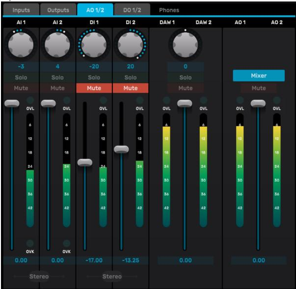
Each input channel has a fader, a high-resolution <u>peak meter</u>, with overload indication 0.05dB below clipping, plus mute and solo buttons and a pan-pot. By engaging the 'Stereo' button beneath an input pair, the pair is controlled by a single stereo fader, mute button and solo button, and the pan-pots are replaced by a single balance control. The DAW contribution and output strip are always in stereo mode.
