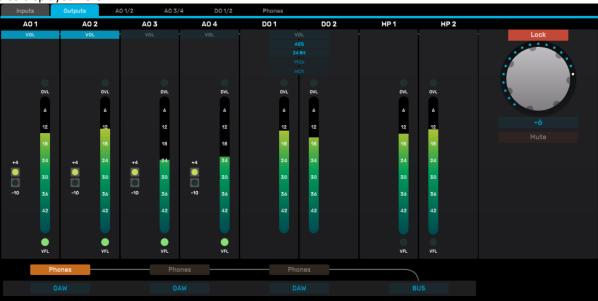
Line output level is switched between +4dBu and -10dBV nominal by the '+4/-10' radio buttons.
