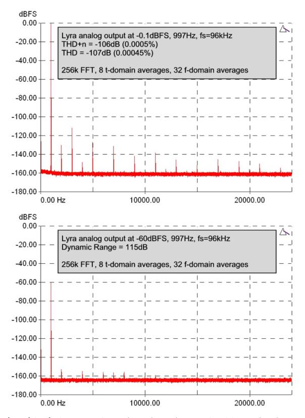
[Note 1]: Specification as per Lyra 2. Lyra 1 does not have analog outputs 3-4, mic input on channel 1, instrument input on channel 2, RCA/phono digital I/O, wordclock I/O or Ethernet port. Lyra 1 SRC THD+n/dynamic range are limited to <-125dB/>125dB (0.000056%) and can only be applied to DI.
