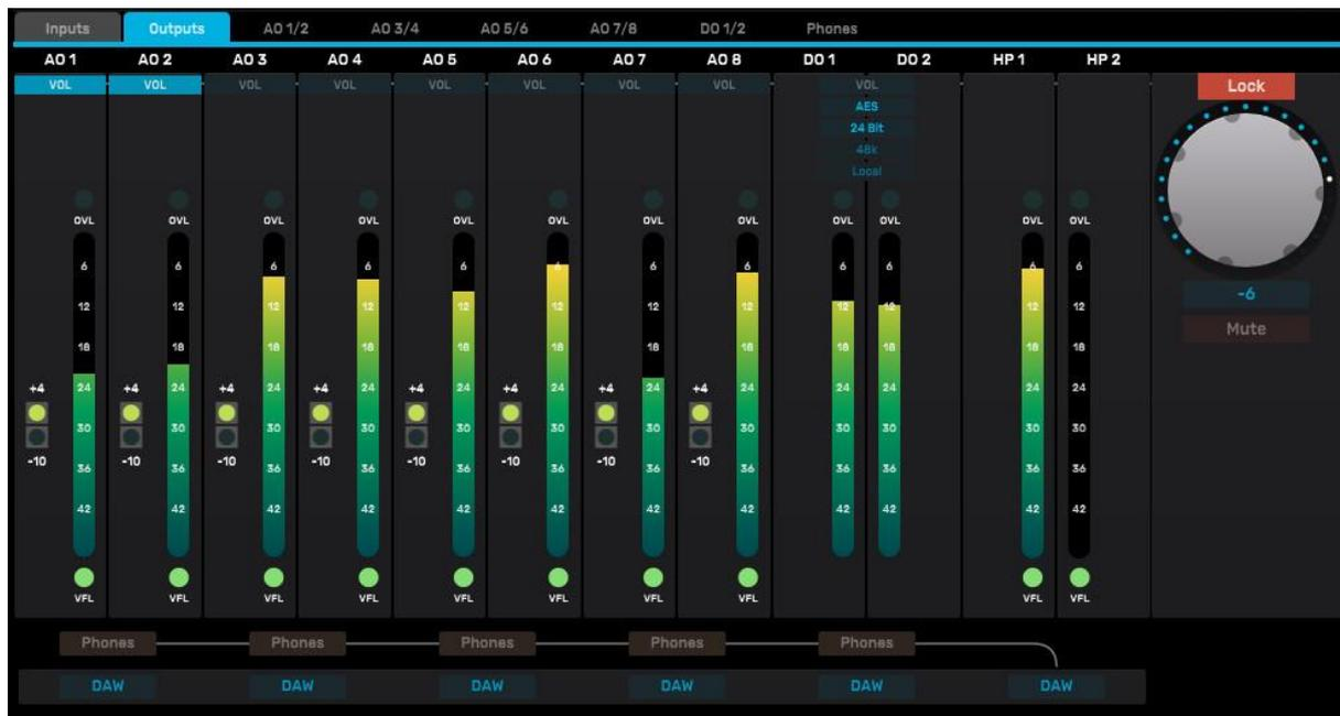
Line output level is switched between +4dBu and -10dBV nominal by the '+4/-10' radio buttons.
