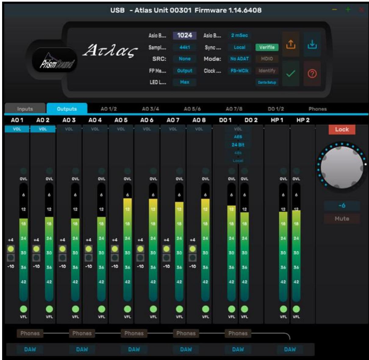
Whilst Atlas can be controlled in a limited way from within the Mac or Windows operating system, or by some audio application programs, most of its detailed features can only be accessed using the Atlas Control Panel app.
