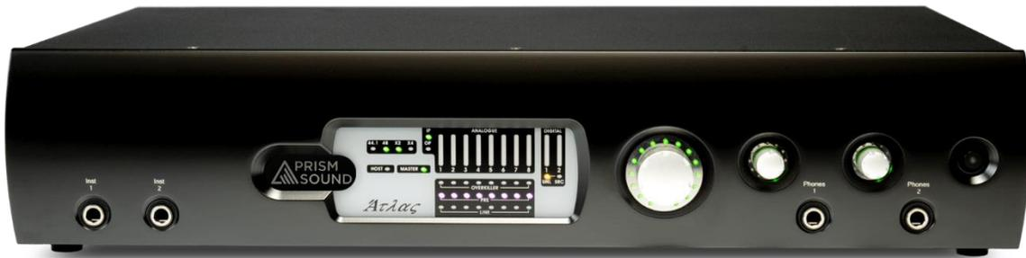
Atlas's front panel contains a limited number of physical controls and indicators. A greater degree of control is available using the [Atlas Control Panel app](#) software provided. The front panel also contains the instrument input and headphone output jacks.
