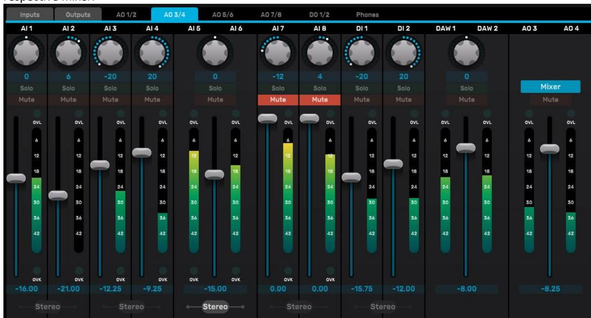
Each input has a fader, a high-resolution [peak meter](#), with overload indication 0.05dB below clipping, plus mute and solo buttons and a pan-pot. By engaging the 'Stereo' button beneath an input pair, the pair is controlled by a single stereo fader, mute button and solo button, and the pan-pots are replaced by a single balance control. The DAW contribution and output strip are always in stereo mode.
